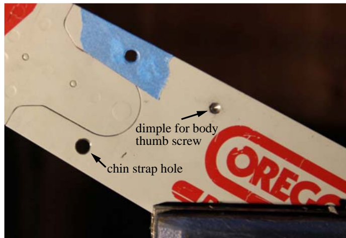
Fig. 2.8. This figure shows a dimple made with a 3/16" Rigid, cobalt, metal-cutting bit. The ball end of the screw seats accurately and reliably in the conical dimple. It is now easy to keep the jig level and at the proper height. I can take the jig off and put it back on and have exactly the same alignment. The jig will not slip down even with the bar coated with oil. Also shown are a pair of 1/4" holes for a chin strap to give the jig some consistent downward pressure.
